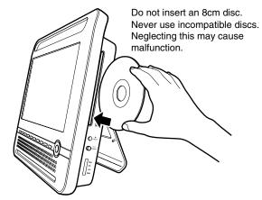
Insert a disc into the disc slot with the label side facing forward. (If the disc has a label.) Hold the disc without touching either of its surfaces, align it with the guides, and place it in position.
